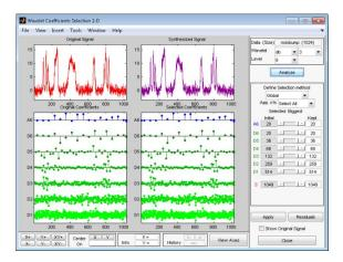
The tool displays below the original signal (on the left) its wavelet decomposition: the approximation coefficients A6 and detail coefficients from D6 at the top to D1 at the bottom. In the middle of the window, below the synthesized signal (which at this step is the same, since all the wavelet coefficients are kept) it displays the selected coefficients.
