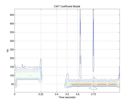
The CWT moduli correctly show the supports of the disjoint sinusoids and the locations of the impulses at 650 and 750 milliseconds. In the CWT moduli, the impulse at 750 milliseconds is clearly visible.
