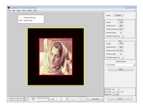
The tool displays the original image delimited by a red box and the transformed image delimited by a yellow box. The image has been extended by zero padding. The right part of the window allows you to control the parameters of the extension/truncation process for the vertical and horizontal directions, respectively. The possibilities are similar to the one-dimensional ones described in "One-Dimensional Extension" on page 2-32.
