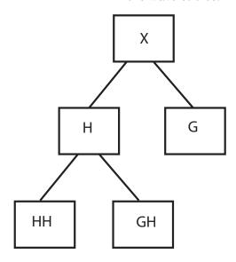
The wavelet packet transform can also operate on the output on the highpass filter. The following figure illustrates one *admissible* binary wavelet packet tree.
